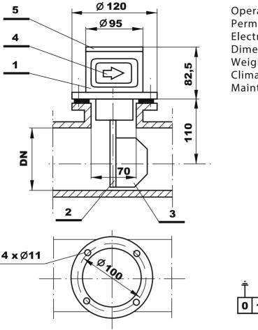
Operating temperature from -30°C to+100°C Permissible gauge pressure in pipeline 4000 hPa Electric contact rating =0,8 A; 220 V Dimension see drawing Weight 1.33 kg Climate no limitation Maintenance no required
